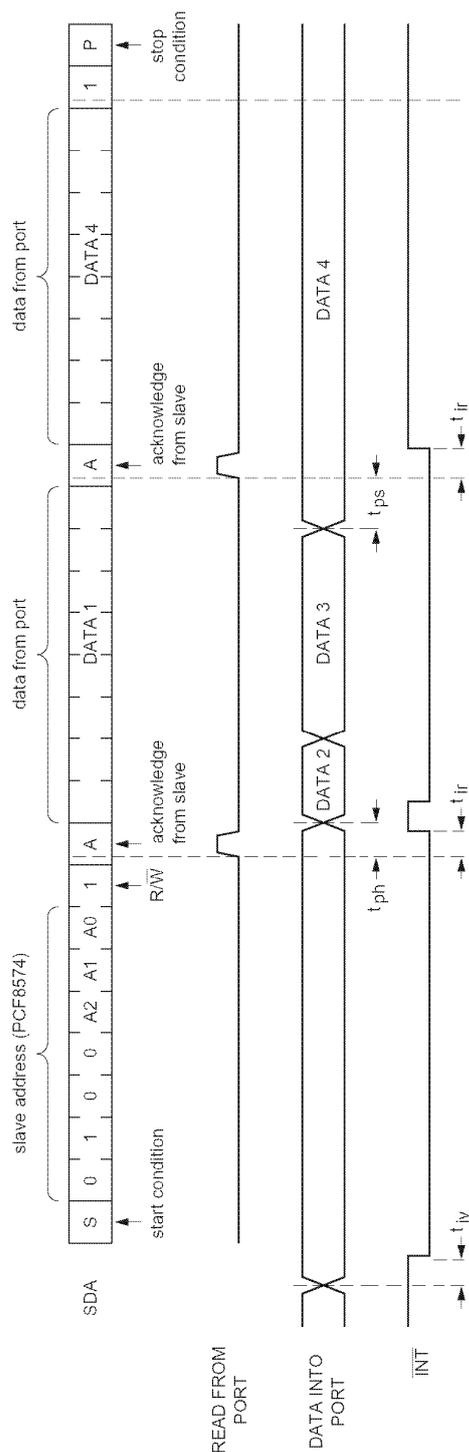
A LOW-to-HIGH transition of SDA, while SCL is HIGH is defined as the stop condition (P). Transfer of data can be stopped at any moment by a stop condition. When this occurs, data present at the last acknowledge phase is valid (output mode). Input data is lost.
